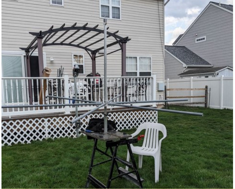
Center post mounted on the spreader plate with 6 the 6 largest spreader elements attached.
