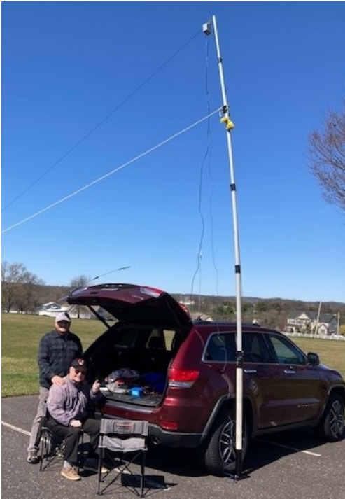
Gene and Griff working 10 Meter AM with a Radio Shack HTX 10 and 40 Meter EFHW
