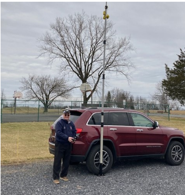
Griff, NE3I checking SWR of his 15 Meter End Fed Half Wave Vertical. QSOs made with stations in Florida, Hawaii, Düsseldorf, Germany, Kansas and Ireland on 15 Meter Phone and CW using only 25 Watts.
