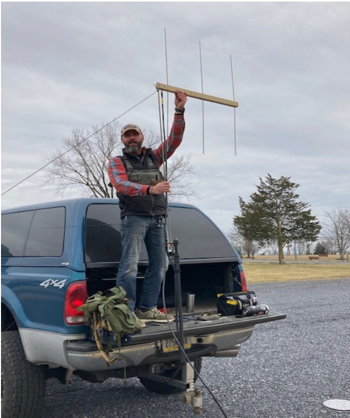
Bryan, W3BFO setting up his "Back Packable" 2 Meter Yagi. The yagi worked well enough to reach out about 8 Miles with 1 Watt.
