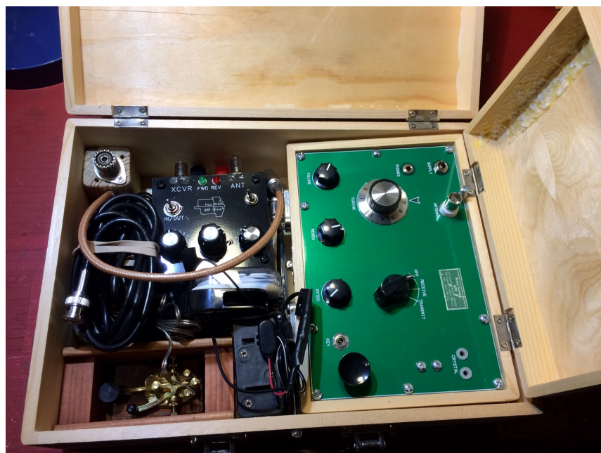
Completed Paraset kit in wooden box with accessories
