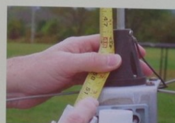
5/8 Wave Length (?) Good SWR at 144.45 Mhz.
