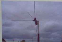
5/8 Wave Length (?) Good SWR at 144.45 Mhz.
