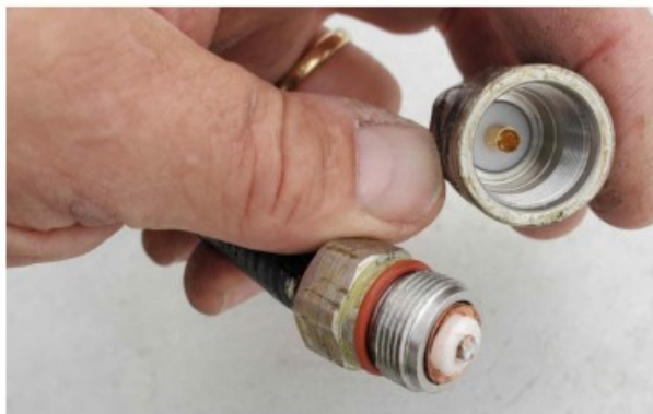
Inside connector showing center conductor pulled back - should be 1/8" into socket.
