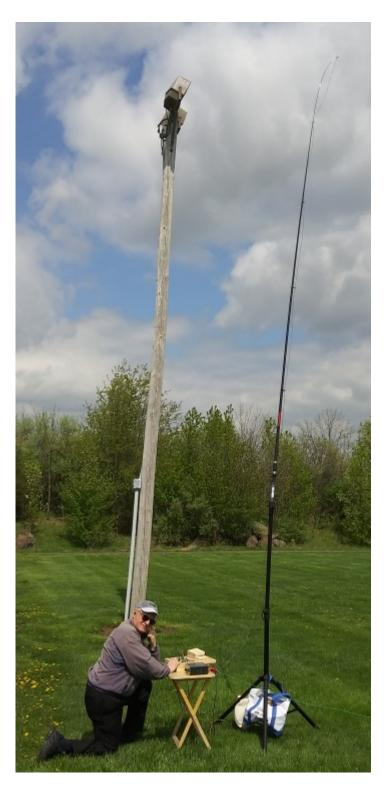
As part of Sunday at the Park Griff NE3I set up a 4W 40M CW rig with a regenerative receiver. He made a contact in Ohio on 7114KHz. This is Dan's fishing pole antenna. Note the green counterpoise wire, a critical part of the antenna system. Photo and technical detail courtesy Dan WA3NFV
